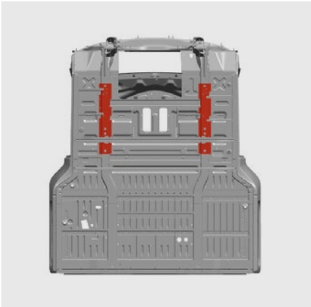
Sled Runners (day cab and sleeper) The HX Series cab variants feature high-strength steel sled runners for improved durability.
