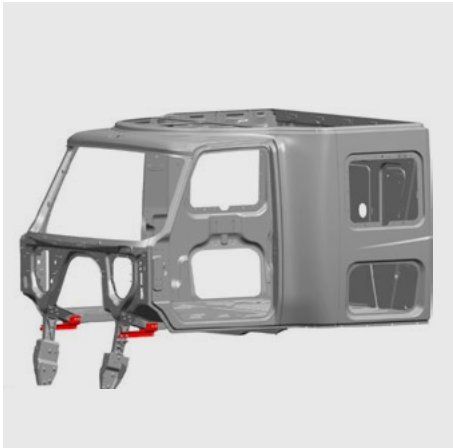
Strut Brace (sleeper only) A strut brace improves dash endurance.
